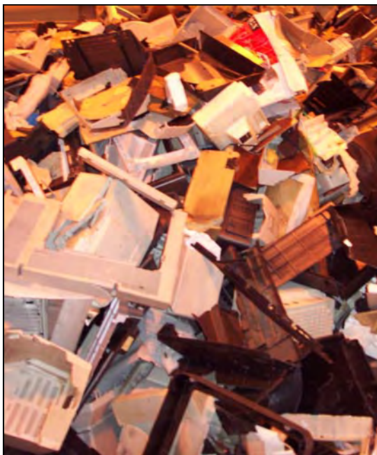
Figur 5 Brominated waste used in the incineration tests (before shredding).
